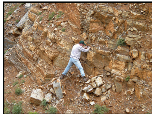
Measuring Strike and Dip on the Chimney Rocks outcrop located adjacent to the Laratonda subdivision property.
